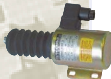
TYPE CI Double coil Pull coil disconnected by external switch Hold coil - ED=100%
