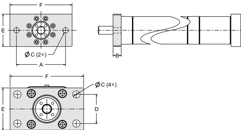
The front mounting plate consists of a plate and comes mounted from the factory if the ordering code states that the unit shall be equipped with one. It can also be ordered as a separate part using the part number in which case it is delivered with the necessary screws to attach it to the actuator.
