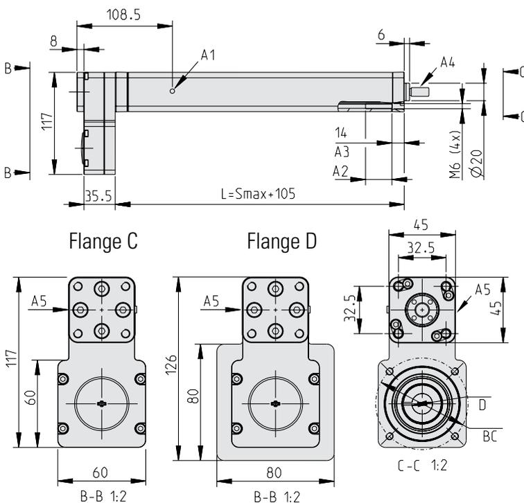
A1: grease port A2: M6 thread, max. depth 30 mm A3: no thread
