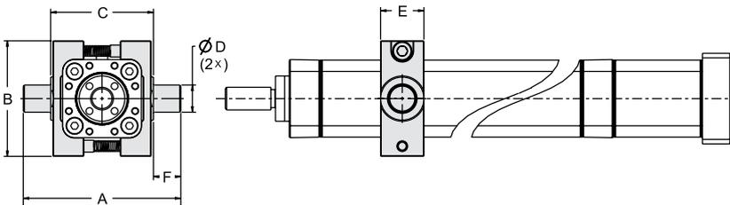
The movable trunnion consists of two clamp units that each have a shaft. The two clamp units are put around the profile of the unit at desired position and joined and locked in place by the lock screws. The movable trunnion comes mounted from the factory if the ordering code states that the unit shall be equipped with one. It can also be ordered as a separate part (all necessary actuator attachment screws are included) using the part number.
