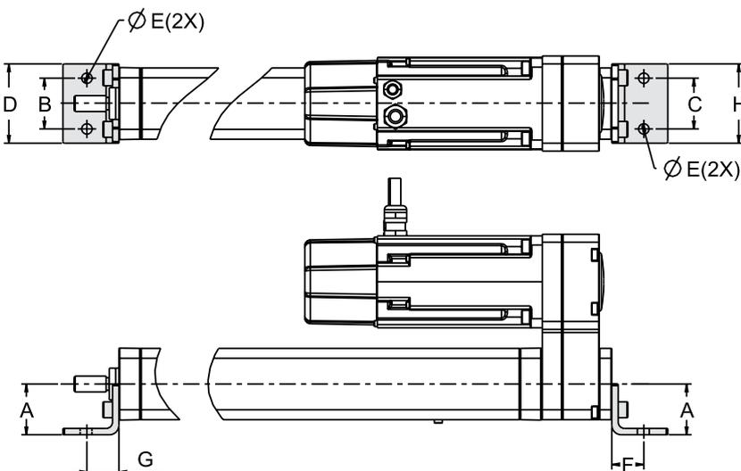
The foot mount consists of a front and rear bracket and comes mounted from the factory if the ordering code states that the unit shall be equipped with one. It can also be ordered as a separate part (all necessary actuator attachment screws are included) using the part number.
