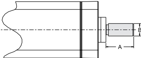
The male threaded rod end comes mounted from the factory if the ordering code states that the unit shall be equipped with one.
