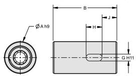
Part number example: GSC25x0500 = glide screw assembly, cylindrical nut, 0.250 inch diameter by 0.500 inch lead
